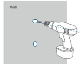
3. Align the holes on the mounting plate with those on the wall, matching the direction as UP and Down indicates. Insert the anchors into the holes; anchors are necessary for walls that are made out of hard materials such as concrete, brick, or stucco. Fix the screws with a Phillips-head screwdriver to fasten the mounting plate onto the wall.
